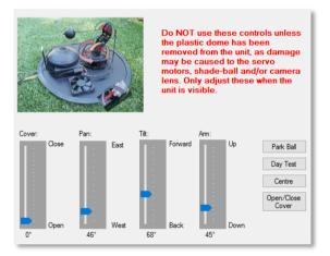
These controls are used to directly adjust the servo motors that control the shade cover and shade-ball's position. They also reflect the current servo angles. As the warning states: **Do NOT use the pan/tilt/arm controls unless the shade cover is open, and the plastic dome has been removed from the unit, as damage may be caused to the servo motors, shade-ball and/or camera lens. Only adjust these when the unit is visible.**
